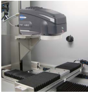
Example of integration on the motorized Z-axis and X/Y table
